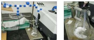
Figure 2: Picture of flow setup and reaction chamber (left). Picture of NaCl+H<sub>2</sub>SO<sub>4</sub> reaction under controlled atmospheric conditions (right)
